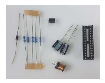
Solder the 5 resistors and the diode first as they are lower profile – its easier to solder the top pad rather than the bottom pad. This prevents the component falling out as you try to solder an inverted PCB! L2 is a tight fit, so push it in hard so that it is as close to the PCBas possible, preventing fouling the top PCB.
