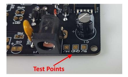
Plug in the power supply, and then test using a DC voltmeter: Touch the black probe on the GND test point and the red probe on the 5V test point. The voltage should measure between 5.6 and 5.9 Volts. If not, disconnect power and check your work. Do not proceed with the assembly until the error is corrected. Once the test is completed, disconnect the power.
