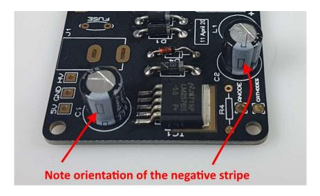
Finally solder the fuse, connector J1 and Inductor L1. L1 is a tight fit, so push it in hard so that it is as close to the PCB as possible, preventing fouling the top PCB.
