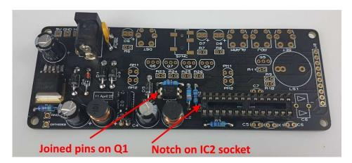
Take care that the notched end of the IC socket is at the end shown. However, if you find you soldered it with the wrong orientation, do not try to remove it. It is perfectly fine with the notch at the wrong end, just be sure to place the IC in the socket with the IC's notch in the correct position.
