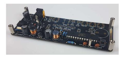
Now push the male and female connectors together and insert the FEMALE side into the J2 position on the main PCB.
