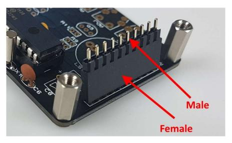
Now lower the upper PCB into place with the pre-soldered IC facing upwards, ensuring the 10 pins are engaged in the 10 holes. Screw in place.
