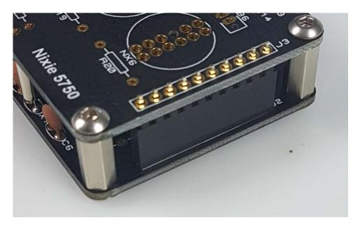
You can now solder all 20 pads, in the knowledge that everything is perfectly alighned. After soldering, remove all the screws and hex spacers and keep them safe for later. Now split the 2 PCBs – it is time to work on the upper tube PCB.
