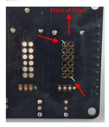
Now solder those 2 pins in place to secure the tube. From above, check the alighnment and orientation of the tube, and make adjustments as necessary by re-wetting the pads until the tube is perfectly front facing and vertical. Then you can solder the remaining 9 pins. Note that one pin is not soldered.
