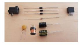
Start by installing D1-D4. The diodes are also polarized – the band on the part must match the band marked on the white PCB marking.
