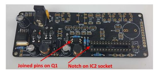
Take care that the notched end of the IC socket is at the end shown. However, if you find you soldered it with the wrong orientation, do not try to remove it. It is perfectly fine with the notch at the wrong end, just be sure to place the IC in the socket with the IC's notch in the correct position.
