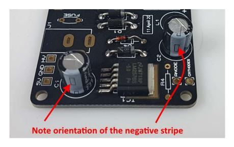
Finally solder the fuse, connector J1 and Inductor L1. L1 is a tight fit, so push it in hard so that it is as close to the PCB as possible, preventing fouling the top PCB.
