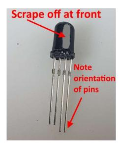
**7.1** Solder each RGB LED in turn – the marking on the PCB indicates the orientation of the longer of the 2 leads. Only 3 leads per LED are soldered.
