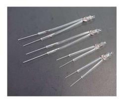
Finally, solder the neons in place on the PCB, with the taller neons at the back.
