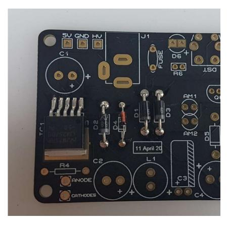
C1 and C2 are polarized. The Positive lead is the longest, and goes in the pad marked `+'.
