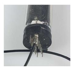
Now, remembering that the board generates 170V, power up the PCB and use the bare end of the cathode wire to touch up against each of the cathode wires in turn, and check that all digits light.
