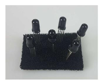
Once dry, scrape a thin band off using a sharp knife. Note the position of the longer 2 pins.
