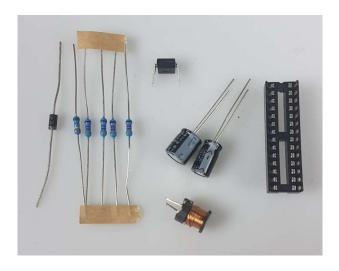
Solder the 5 resistors and the diode first as they are lower profile – its easier to solder the top pad rather than the bottom pad. This prevents the component falling out as you try to solder an inverted PCB! L2 is a tight fit, so push it in hard so that it is as close to the PCBas possible, preventing fouling the top PCB.
