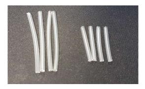
Slip the insulation over the neon lamp leads and with a hot air gun, shrink the tubing:
