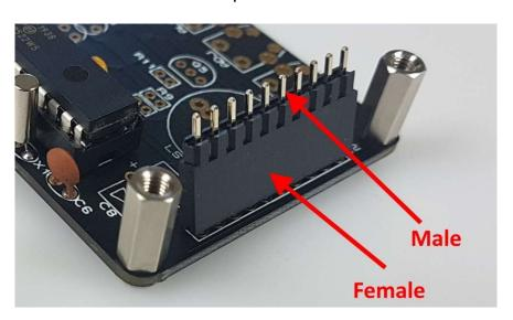
Now lower the upper PCB into place with the pre-soldered IC facing upwards, ensuring the 10 pins are engaged in the 10 holes. Screw in place.
