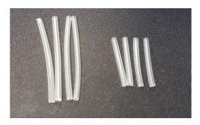
Slip the insulation over the neon lamp leads and with a hot air gun, shrink the tubing:
