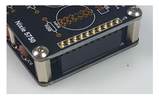
You can now solder all 20 pads, in the knowledge that everything is perfectly alighned. After soldering, remove all the screws and hex spacers and keep them safe for later. Now split the 2 PCBs – it is time to work on the upper tube PCB.
