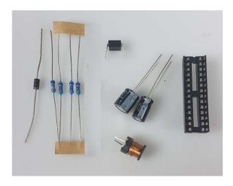
Solder the 4 resistors and the diode first as they are lower profile – its easier to solder the top pad rather than the bottom pad. This prevents the component falling out as you try to solder an inverted PCB! L2 is a tight fit, so push it in hard so that it is as close to the PCB as possible, preventing fouling the top PCB.
