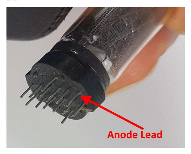
Then, push the anode test lead, with the socket on, onto the anode lead.
