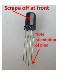
**7.1** Solder each RGB LED in turn – the marking on the PCB indicates the flat on the LED body. Only 3 leads per LED are soldered.
