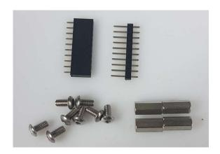
Start by screwing the 11mm hex spacers to each corner of the main PCB:
