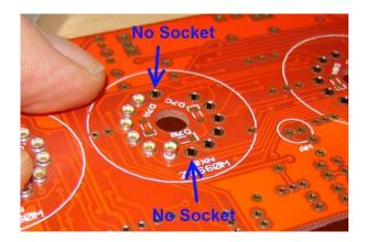
The flip the PCB over, and press the socket firmly into position against a hard surface:
