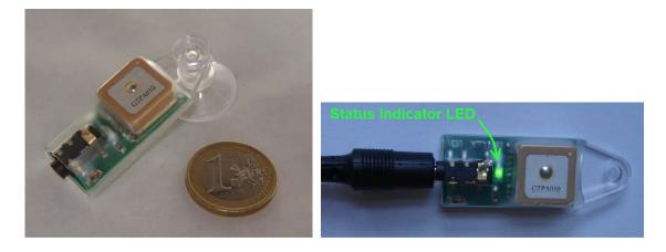
The GPS Sync module outputs data at 4,800 bps in a RS232 format.
