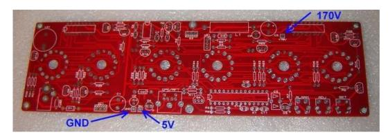
Plug in the power supply, and then test using a DC voltmeter: Touch the black probe on the GND test point and the red probe on the 5V test point. The voltage should measure between 4.9 and 5.1 Volts. If not, disconnect power and check your work. Do not proceed with the assembly until the error is corrected. Once the test is completed, disconnect the power.
