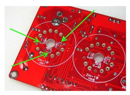
Now identify the cathode mark on the LEDs. This is usually a green marking at one end of the LED, though it may be under the LED lens and harder to see, It may also be an arrow or a line pointing in one direction on the underside of the LED:
