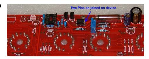
Take care that the two pins that are joined go in the position marked. C5 and C8 are polarised. The longer lead goes in the '+' hole.
