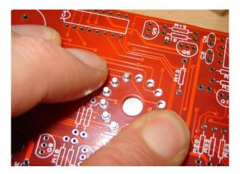
Be sure to insert the sockets FROM the tube side of the PCB – the side with the tube markings. Then solder each socket in place.
