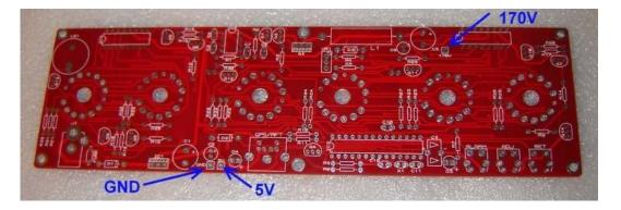
Plug in the power supply, and then test using a DC voltmeter: Touch the black probe on the GND test point and the red probe on the 5V test point. The voltage should measure between 4.9 and 5.1 Volts. If not, disconnect power and check your work. Do not proceed with the assembly until the error is corrected. Once the test is completed, disconnect the power.
