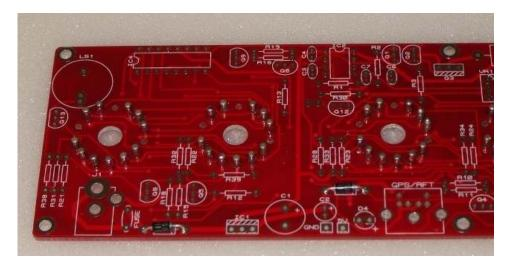
Proceed to mount the other components of this step. Capacitor C1 is polarised: the longer lead goes in the hole marked `+'. C2 is not polarised. Keep IC1 mounted vertical for the moment. It can be bent over to lower the profile of the board at the end of assembly.
