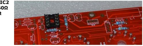
Socket for IC2 R1, R2 - 560Ω R4 - 620ΚΩ R5 - 4.3ΚΩ 4.4 Q1 - BC639 Q2 - BC640 C3 - 330pF C4 - 100nF C7 - 100nF
