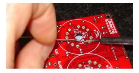
Using tweezers, place the LED over its pads and re-apply the soldering iron briefly to the pad with the solder on. This will re-melt the solder and anchor the LED. Now solder the other pad of the LED.
