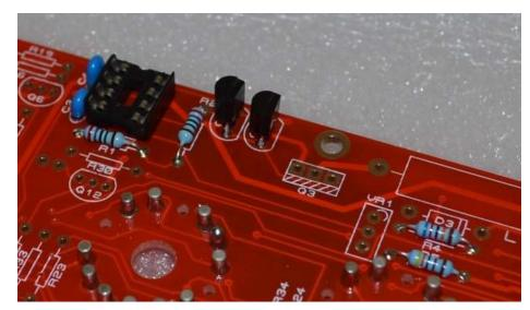
Note, that C7 is mounted on the TUBE side of the PCB, directly across pins 4 and 5 of IC2:
