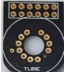
**CD66, ZM1240 and ZM1242:** These tubes have 1 lead at the very back of the tube that needs to be removed. Ensure you only clip the lead at the very back of the tube, this will leave you with 11 leads remaining and a gap at the back of the tube. Proceed as for XN11 and XN12 below.
