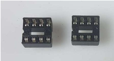
Note: Earlier versions of the kit may not have the sockets – its perfectly safe to solder Q2 to Q5 directly to the PCB.
