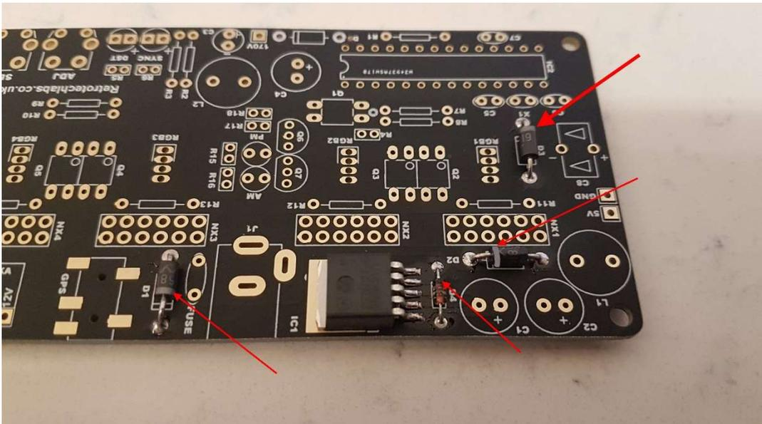
Continue to mount C1, C2, L1, J1 and FUSE. C1 and C2 are polarized. The longer lead goes in the hole marked '+'.
