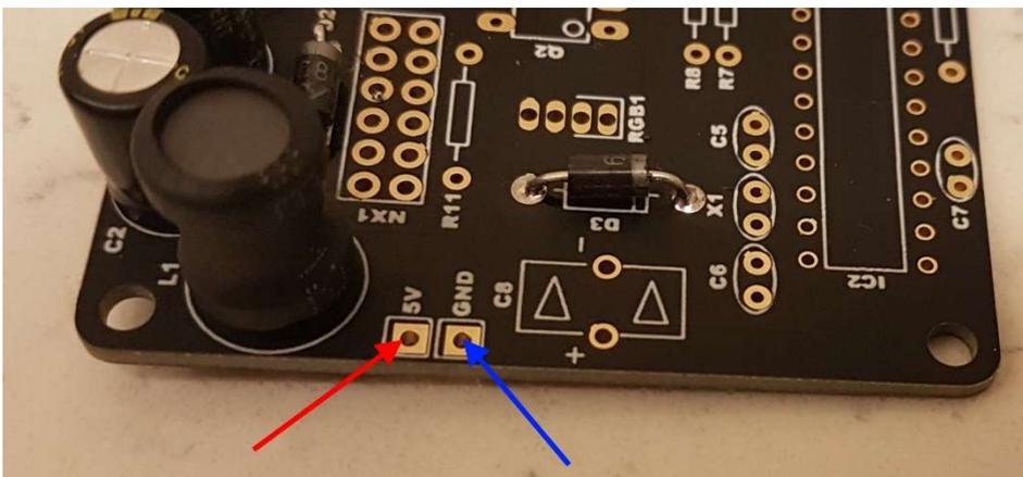
Plug in the power supply, and then test using a DC voltmeter: Touch the black probe on the GND test point and the red probe on the 5V test point. The voltage should measure between 5.4 and 5.8 Volts. If not, disconnect power and check your work. Do not proceed with the assembly until the error is corrected. Once the test is completed, disconnect the power.
