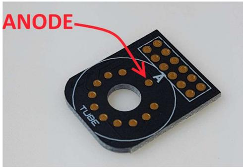
Now you can insert and solder in the tube. Pay attention that the tube sits squarely on the PCB. Then solder on the connector.
