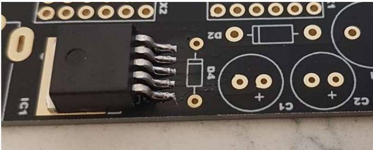
Now solder the four diodes, taking care that the band on the diode matches the band marked on the PCB as shown below.
