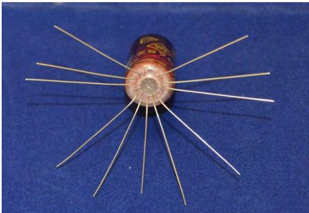
To facilitate easy insertion of the flying leads into the PCB holes, it helps enormously to trim the remaining flying leads with a pair of scissors as shown below. Start at one of the leads at the back of the tube.
