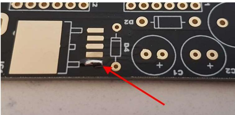
Now place the part IC2 over the soldered pad. Ensure the part is
