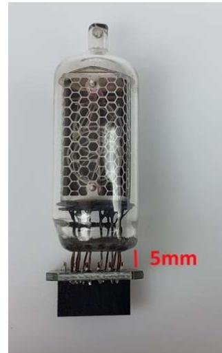
The tube cell is now complete. Repeat for the other 3 tubes. Then move on to step 6.
