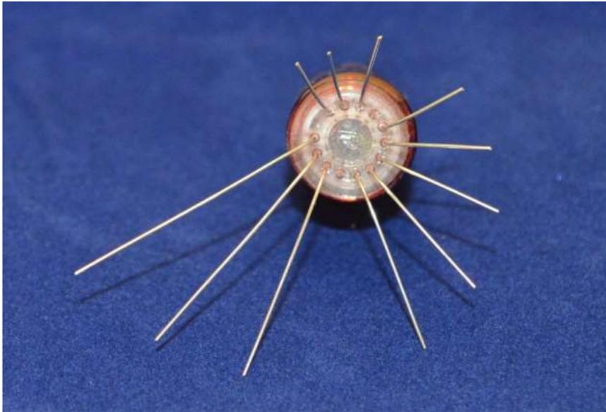
Now you can insert and solder in the tube. There are 11 leads on the trimmed tube and 12 pads on the PCB. One of the pads on the PCB is unconnected. DO NOT INSERT A LEAD INTO THIS HOLE:
