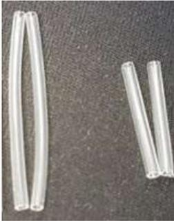
Slip the insulation over the neon lamp leads and with a hot air gun, shrink the tubing:
