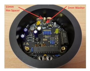
Adjust the Sync LED, D6 so it points towards the hole in the side of the case.
