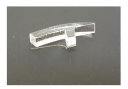
Push the lens into place – the stem goes into the hole in the side of The case, which the Sync LED D6 shines through.
