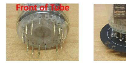
Then insert the tube into the PCB, engaging the 11 gold sockets into the 11 sockets soldered to the PCB. Solder the gold sockets to the PCB sockets.
