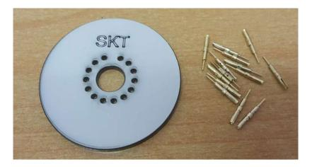
Remove the protective film from both sides, and insert all the sockets into the socket holder from the side engraved 'SKT'. Insert the socket with the open jaws first. You may need to push each socket in firmly, with a hard object. Also solder the 6X2 FEMALE connector to the tube PCB. This is what you end up with:
