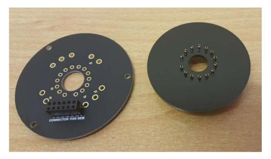
Now you can push the socket holder into the PCB firmly and fully, and solder in place:
