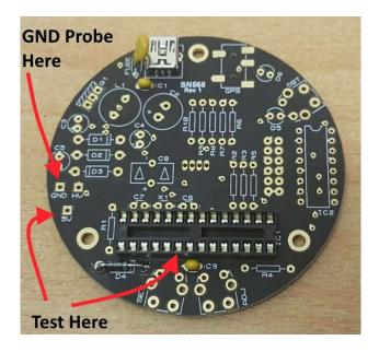
The voltages should measure between 4.9 and 5.2 Volts. If not, disconnect power and check your work. Do not proceed with the assembly until the error is corrected. Once the test is completed, disconnect the power.
