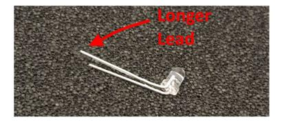
D5 and D6 are polarised. The longer lead is the positive (anode) and goes in the holes marked below.
