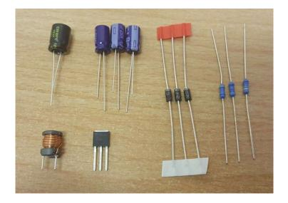
Orient the diodes with the white band matching the corresponding band on the PCB. Also the capacitors are polarised. The longer, positive lead for each goes in the hole marked below.
