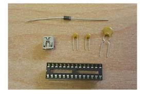
C1 and C9 will be marked `104'. Align the band on D4 with the band marked on the PCB. Orient the notch on the IC socket with the corresponding marking on the PCB.
