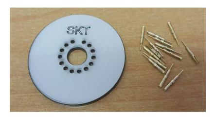
Remove the protective film from both sides, and insert all the sockets into the socket holder from the side engraved 'SKT'. Insert the socket with the open jaws first. You may need to push each socket in firmly, with a hard object. Also solder the 6X2 FEMALE connector to the tube PCB. This is what you end up with:
