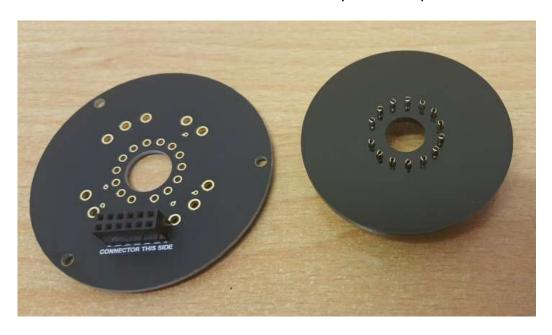
Now you can push the socket holder into the PCB firmly and fully, and solder in place:
