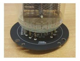
Then insert the tube into the PCB, engaging the 11 gold sockets into the 11 sockets soldered to the PCB. Solder the gold sockets to the PCB sockets.
