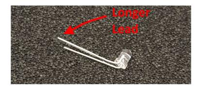
D5 and D6 are polarised. The longer lead is the positive (anode) and goes in the holes marked below.
