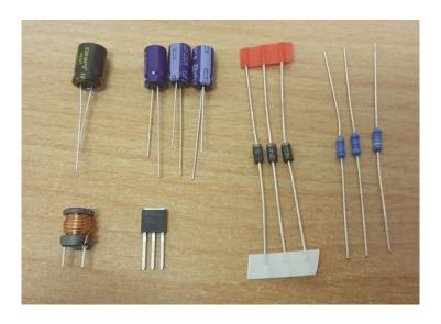
Orient the diodes with the white band matching the corresponding band on the PCB. Also the capacitors are polarised. The longer, positive lead for each goes in the hole marked below.
