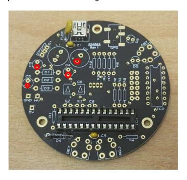
Do not solder Q1 fully flush with the PCB. It is best for it to be 5mm or so from the PCB, so you are not soldering so close to the body of the part, so less heat will reach the part.
