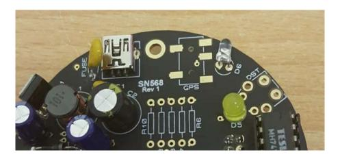
Note that D6 points sideways, as it will shine through the corresponding hole in the case. If you are making your own case, you can solder both LEDs differently.
