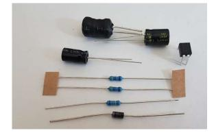
Take care that you have the correct part for Q1. It has 2 of its pins joined as they come out of its black resin body. Also the MOSFET needs to be placed with the two joined pins as marked on the PCB.
