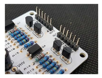
Also solder the 4 way headers at the DEK1 DEK2 positions where you will use jumpers to select which of three modes each Dekatron operates in. It helps to put the jumpers onto the pins before soldering, so the pins are in exactly the right place.
