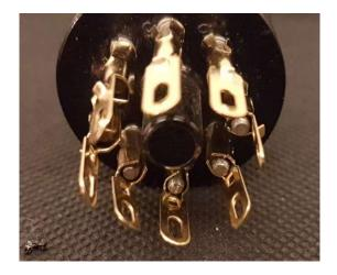
Now gently feed the sockets into the matching slots on the tube PCB. Get the alignment of the tube correct with regard to the slot on the PCB. Be really careful to push the tube in from the correct side of the PCB, marked 'Tube Side'. Then solder the sockets. Don't flood with too much solder that the solder passes through the PCB and solders the actual tube pin!
