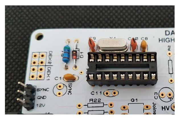
4.5 High Voltage Generator components. R2, R3 (4.7 KΩ) R4 (390 KΩ) C2 (220uF) C3 (1uF) D2 (UF4004) Q1 (IRFD220) L1 (100uH Inductor)
