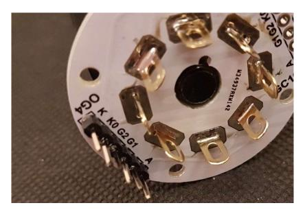
Use two 3-Way cables to connect up the tube to the driver PCB. Use the different colours of the cables to ensure the connections match!
