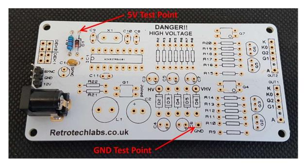
Plug in the 12V DC power supply, and then test using a DC voltmeter: Touch the black probe on the GND test point and the red probe on the 5V test point. The voltage should measure between 5.4 and 5.8 Volts. If not, disconnect power and check your work. Do not proceed with the assembly until the error is corrected. Once the test is completed, disconnect the power. **IF YOU CHOOSE TO PROCEED BEYOND THIS POINT WITHOUT GETTING THE CORRECT VOLTAGE, WE WILL NOT BE ABLE TO OFFER SUPPORT**
