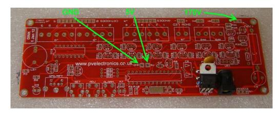
Plug in the power supply, and then test using a DC voltmeter: Touch the black probe on the GND test point and the red probe on the 5V test point. The voltage should measure between 5.3 and 5.7 Volts. If not, disconnect power and check your work. Do not proceed with the assembly until the error is corrected. Once the test is completed, disconnect the power.
