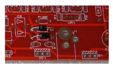
**4.2** Continue to mount IC1 with D5 attached. After placement, IC1 can be placed and bent over to reduce the height of the assembled PCB. The fuse and J1 may now be placed in position.
