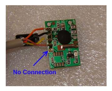
Now attach the antenna by soldering the two antenna wires to the pads marked 'ANT':
