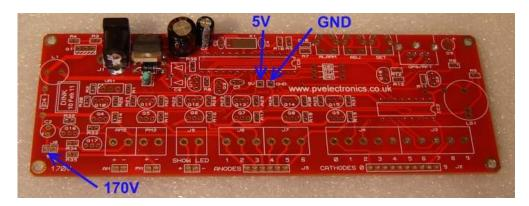
Plug in the power supply, and then test using a DC voltmeter: Touch the black probe on the GND test point and the red probe on the 5V test point. The voltage should measure between 5.1 and 5.3 Volts. If not, disconnect power and check your work. Do not proceed with the assembly until the error is corrected. Once the test is completed, disconnect the power.
