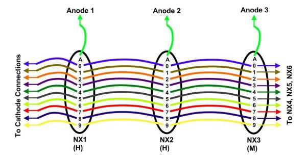
There will be just 16 wires from the tubes leading back to the PCB (10 for the cathodes and 6 for the anodes). Connect to either the screw terminals or the pin headers (via sockets / pins if you wish)
