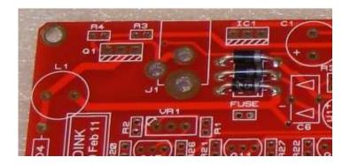
After placement, IC1 can be placed and bent over these diodes to reduce the height of the assembled PCB. Continue to mount C1, C2, J1 and FUSE. Note that C1 and C2 are polarised. The longer lead goes in the hole marked (+).
