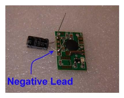
Then clip the excess capacitor leads so there is only 1-2mm remaining.
