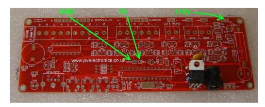
Plug in the power supply, and then test using a DC voltmeter: Touch the black probe on the GND test point and the red probe on the 5V test point. The voltage should measure between 4.9 and 5.1 Volts. If not, disconnect power and check your work. Do not proceed with the assembly until the error is corrected. Once the test is completed, disconnect the power.
