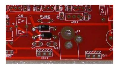
Continue to mount IC1. After placement, IC1 can be placed and bent over to reduce the height of the assembled PCB. The fuse and J1 may now be placed in position.
