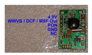
Note that one pad marked is not connected (NC). We recommend connecting a 100uF electrolytic capacitor across the 4.8V and GND pads as close as possible to the module. There are no special requirements for the cable used: light duty 4-way signal cable is suitable for making the connections.
