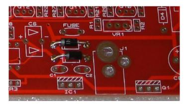
**4.2** Continue to mount IC1 with D5 attached. After placement, IC1 can be placed and bent over to reduce the height of the assembled PCB. The fuse and J1 may now be placed in position.
