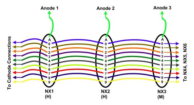
There will be just 16 wires from the tubes leading back to the PCB (10 for the cathodes and 6 for the anodes). Connect to either the screw terminals or the pin headers (via sockets / pins if you wish)
