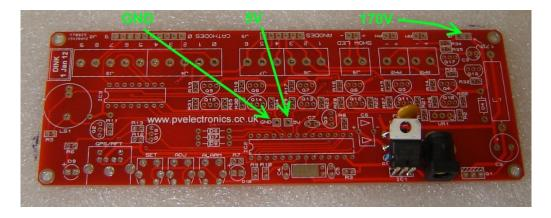
Plug in the power supply, and then test using a DC voltmeter: Touch the black probe on the GND test point and the red probe on the 5V test point. The voltage should measure between 5.3 and 5.7 Volts. If not, disconnect power and check your work. Do not proceed with the assembly until the error is corrected. Once the test is completed, disconnect the power.
