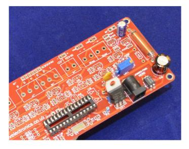
If your kit contains the radial inductor, use a short piece of wire to extend one lead of the inductor as shown below:
