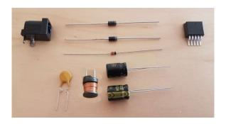
IC1 is a Surface Mount part, but it is large and easy to solder. Start by wetting one pad with solder. Then place the part in position and heat the lead so the solder below it melts and anchors the part. The four other leads can then be soldered. Do not solder the heatsink tab.
