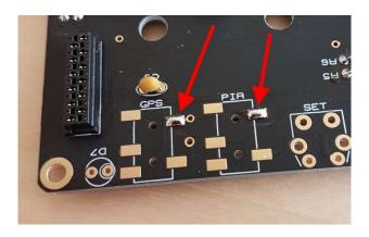
Then place the socket over the pad and re-heat the pad to wet the solder and anchor the part. The remaining pads can then be soldered.
