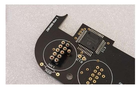
Solder sparingly – as soon as you see solder flow around the annulus, withdraw the solder and soldering iron.
