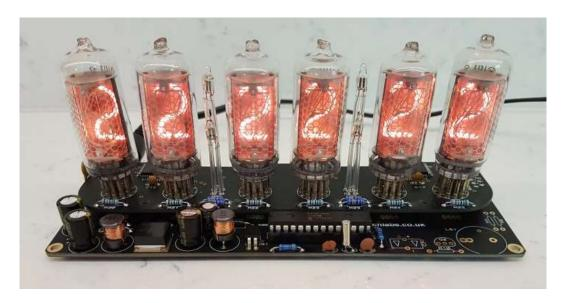
If you do not get this count UP, or have missing or overlapping digits, stop and check your work. Missing digits is usually rectified by pinching the tube contacts (when powered off!) so they make better contact with the tube. Also try swapping tubes around to see if the problem is with the tube, or the location. Please make these basic tests before contacting us for help and have the results to hand.
