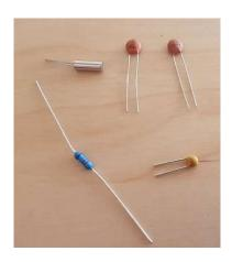
The 10pF capacitor is usually marked '15' and not surprisingly the 33pF is marked '33'. The 100nF is marked 104. Don't switch C5 and C6 or the timekeeping will be very slow.
