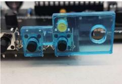
Now bend and solder D7. The longer lead goes in the pad with a circle around it. Think about the orientation before you bend the leads. D7 should be level with the GPS jack socket next to it, and protrude by its full body length from the rear of the PCB.
