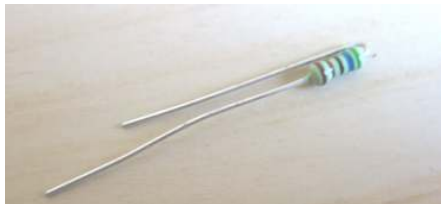
Figure 7: Resistor leads formed for mounting upright.
