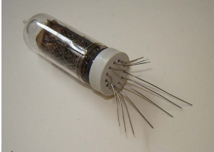
Figure 16: IN-14 flying leads trimmed to aid insertion into the PCB
