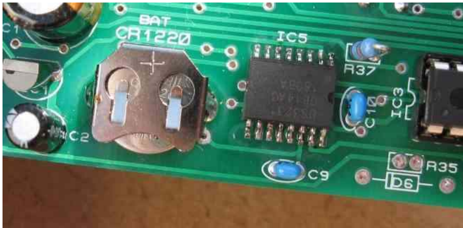
Figure 24: Showing all RTC components: IC5, C9, C10, Lithium Cell
