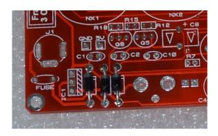
After placement, IC1 can be placed and bent over these diodes to reduce the height of the assembled PCB. Continue to mount C1, C2, J1 and FUSE.
