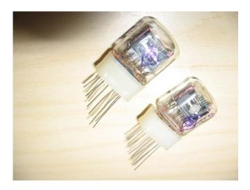
Be aware that each tube has one wire 'missing'. The tube is manufactured this way.
