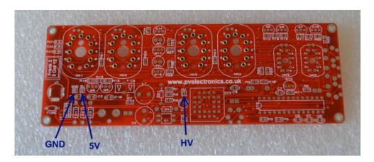
Plug in the power supply, and then test using a DC voltmeter: Touch the black probe on the GND test point and the red probe on the 5V test point. The voltage should measure between 5.5 and 5.9 Volts. If not, disconnect power and check your work. Do not proceed with the assembly until the error is corrected. Once the test is completed, disconnect the power.
