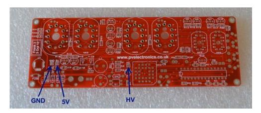
Plug in the power supply, and then test using a DC voltmeter: Touch the black probe on the GND test point and the red probe on the 5V test point. The voltage should measure between 5.1 and 5.3 Volts. If not, disconnect power and check your work. Do not proceed with the assembly until the error is corrected. Once the test is completed, disconnect the power.
