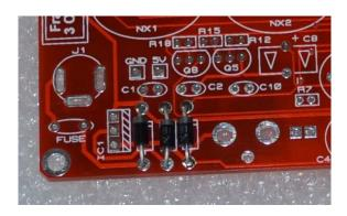
After placement, IC1 can be placed and bent over these diodes to reduce the height of the assembled PCB. Continue to mount C1, C2, J1 and FUSE.
