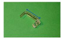
Now bend again, appropriate to the spacing between the pads for the LED and the hole for the LED. Cut the leads to the same length:
