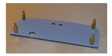
Then place the tube PCB over the four studs and place a 2mm washer over each stud:
