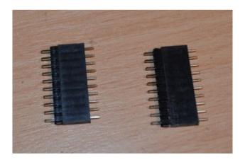
Place the connectors into the main component PCB with the male connector in this PCB, so that when you place the tube PCB over the top, the female connectors go into the holes on the tube PCB.
