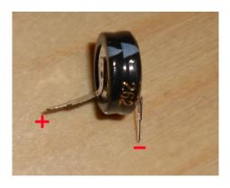
Solder the (-) lead into the hole on the COMPONENT side of the PCB as shown below. Do not insert the (+) lead into the other hole. This should be connected to the banded end of D3 as shown below:
