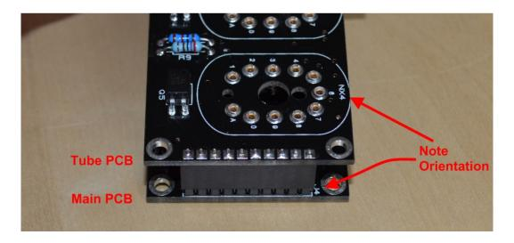
Ensure the two PCBs are perfectly square and true, and then solder all the connectors in place. It is a good idea to solder the four top corner pins in place and then the four bottom corner pins first, so the connectors are anchored. Then you can solder all the remaining pins. After soldering, the PCBs can be split into 2 parts again.
