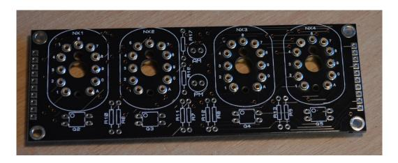
Then place a hard flat object over the sockets and flip over the PCB and solder the sockets in place as shown below:
