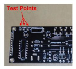
Plug in the power supply, and then test using a DC voltmeter: Touch the black probe on the GND test point and the red probe on the 5V test point. The voltage should measure between 5.1 and 5.3 Volts. If not, disconnect power and check your work. Do not proceed with the assembly until the error is corrected.
