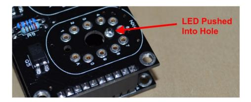
Turn the PCBs over so you can solder the LEDs in place, ensuring they are pushed completely into the holes in the tube PCB. The two PCBs may now be pulled apart for the rest of the assembly.
