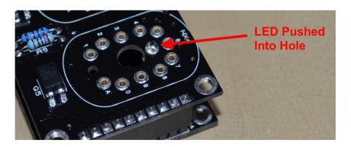
Turn the PCBs over so you can solder the LEDs in place, ensuring they are pushed completely into the holes in the tube PCB. The two PCBs may now be pulled apart for the rest of the assembly.
