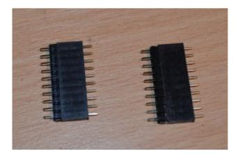
Place the connectors into the main component PCB with the male connector in this PCB, so that when you place the tube PCB over the top, the female connectors go into the holes on the tube PCB.
