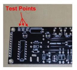
Plug in the power supply, and then test using a DC voltmeter: Touch the black probe on the GND test point and the red probe on the 5V test point. The voltage should measure between 5.5 and 5.8 Volts. If not, disconnect power and check your work. Do not proceed with the assembly until the error is corrected.
