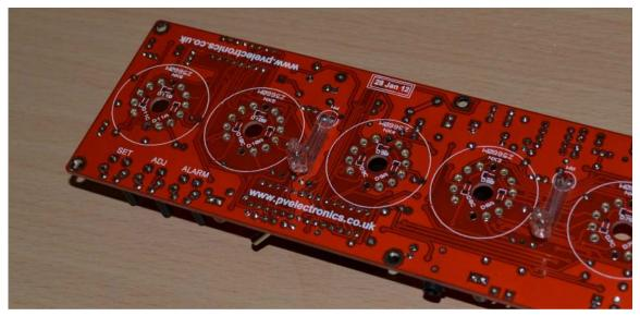
Note that the neons are mounted nearer to the bottom edge of the PCB, which is the edge where the switches and power socket are.
