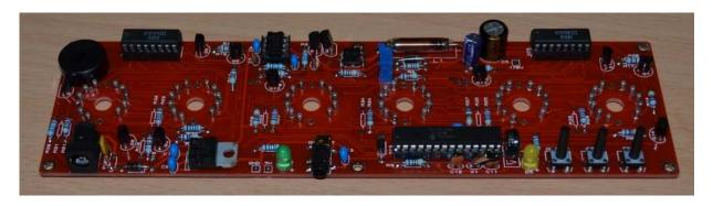
The longer lead of each LED goes in the hole marked '+'.
