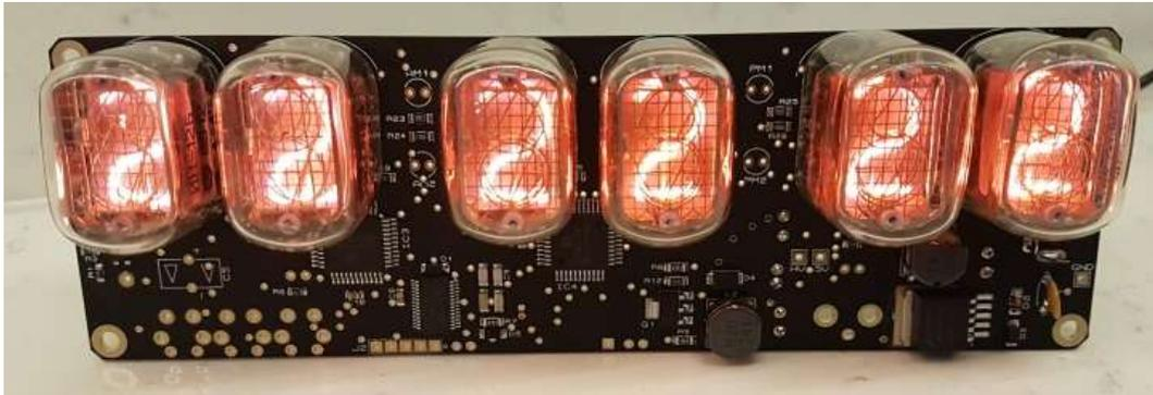
If you do not get this count up, or have missing or overlapping digits, stop and check your work. Try swapping tubes around to see if the problem is with the tube, or the location. Please make these basic tests before contacting us for help and have the results to hand. If no tubes light, check the 5V and HV test points with your multimeter, with the black probe on the GND test point. The 5V test point should measure 5.3V to 5.9V and the HV test point 165V to 178V.
