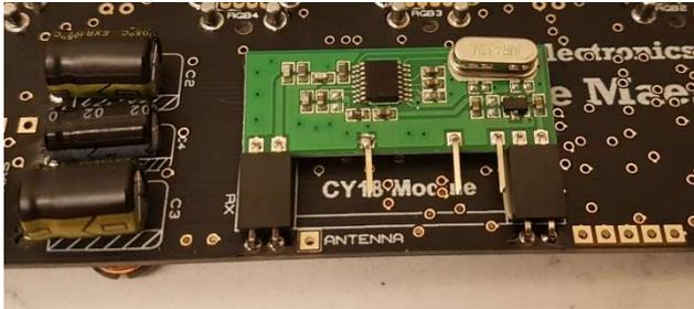
Finally, measure out exactly 17cm of the antenna wire cable, strip off 2mm from one end and solder to the ANTENNA Pad. This Antenna wire can be routed conveniently and neatly inside the final enclosure you make or buy.
