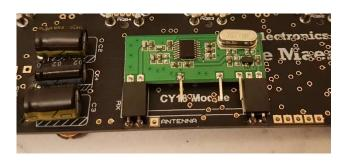
Finally, measure out exactly 17cm of the antenna wire cable, strip off 2mm from one end and solder to the ANTENNA Pad. This Antenna wire can be routed conveniently and neatly inside the final enclosure you make or buy.
