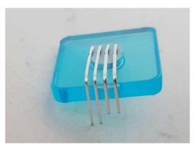
Then install the RGB LEDs from the back of the PCB, and solder from the front of the PCB. Clip off the excess leads.
