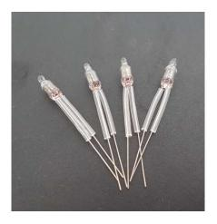
The four neons can now be soldered onto the PCB.
