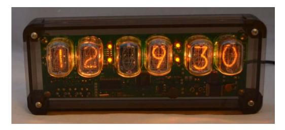
Red = 9, therefore Auto Colour Cycling is enabled for 12-13 hours. Green = 3, so speed is 3. Blue value has no effect.
