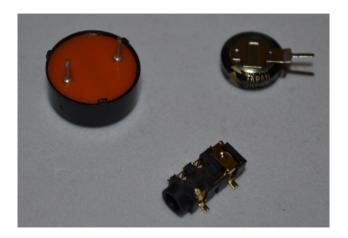
To solder the GPS / RFT connector: First wet one pad on the PCB with solder. Then place the connector in position and re-touch the pad with the soldering iron. This will anchor the component and then you can solder the remaining pads.
