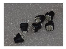
Install an LED at each LED location, looking carefully for the 'notched' corner on each LED which is partially masked by the heat shrink, but still visible. This aligns with a corresponding PCB mark . Solder in each LED and then the other components of this step:
