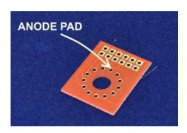
NOTE: IN-14 Cells supplied from August 2013 will not have the two holes either side of the anode. Simply clip off the two leads either side of the anode.
