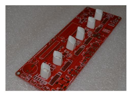
**4.4** Using the hot air gun or hairdryer, GENTLY shrink the tubing over the LEDs Using low heat setting and keep the gun far from the PCB and keep moving. Rotate the PCB to shrink the back of the tubing as well. Then let the PCB cool for 2 minutes at is will be quite warm. It should now look like this:
