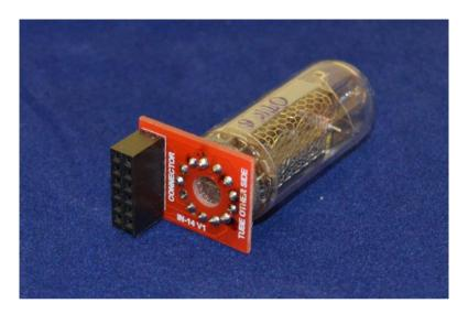
The tube cell is now complete. Repeat for the other 5 tubes. Then move on to step 7.
