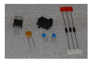
Start by installing D1-D3. Align the white band on the components with the band marked on the PCB. After placement, IC1 can be placed and bent over these diodes to reduce the height of the assembled PCB. Continue to mount C1, C2, J1 and FUSE.
