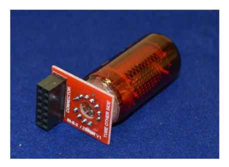
The tube cell is now complete. Repeat for the other 5 tubes. Then move on to step 7
