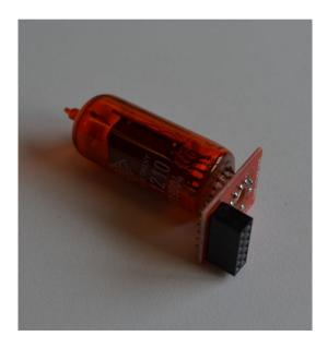
The tube cell is now complete. Repeat for the other 5 tubes. Then move on to step 7.
