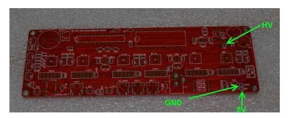
Plug in the power supply, and then test using a DC voltmeter: Touch the black probe on the GND test point and the red probe on the 5V test point. The voltage should measure between 5.1 and 5.3 Volts. If not, disconnect power and check your work. Do not proceed with the assembly until the error is corrected. Once the test is completed, disconnect the power.
