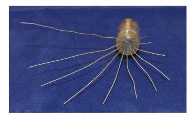
Now you can insert and solder in the tube. Insert the 12 leads into the 12 holes. Insert from the side of the PCB with no markings. Pay attention that the tube sits squarely on the PCB. Ensure the tube is facing perfectly forwards before soldering - you may need to twist it a little.
