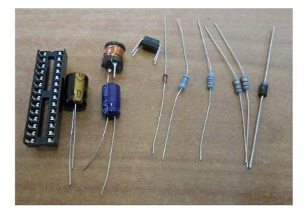
All the resistors on the board need to be mounted upright to save space. The leads need to be formed as shown below. Bend the leads of each resistor as shown and solder in to the correct postion, making sure the component body is as close to the board as possible.
