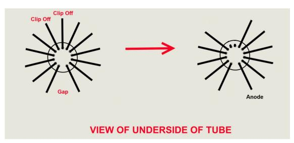
To facilitate easy insertion of the flying leads into the small holes, it helps enormously to trim the flying leads with a pair of scissors. Start at one of the leads at the back of the tube. Then, working around the tube, cut each successive lead approx 2mm shorter than the previous one. This will allow you to feed each lead in in turn.
