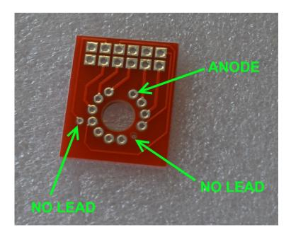
Pay attention that the tube sits squarely on the PCB. Ensure the tube is facing perfectly forwards before soldering - you may need to twist it a little.
