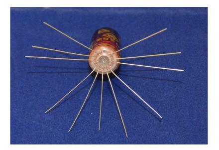
To facilitate easy insertion of the flying leads into the PCB holes, it helps enormously to trim the remaining flying leads with a pair of scissors as shown below. Start at one of the leads at the back of the tube. Then, working around the tube, cut each sucessive lead approx 2mm shorter than the previous one. This will allow you to feed each lead in in turn.
