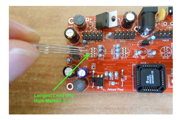
Then, place a Nixie Tube assembly into position on the 6X2 connectors. Push the RGB LED gently into position under the tube and then solder in place:
