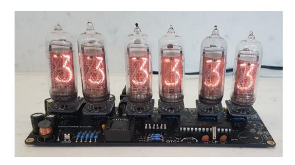
If you do not get this count up, or have missing or overlapping digits, stop and check your work. Try swapping tubes around to see if the problem is with the tube, or the location. Please make these basic tests before contacting us for help and have the results to hand.
