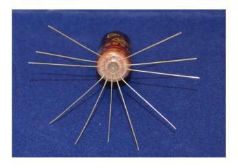
To facilitate easy insertion of the flying leads into the PCB holes, it helps enormously to trim the remaining flying leads with a pair of
