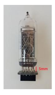
The tube cell is now complete. Repeat for the other 5 tubes. Then move on to step 6.
