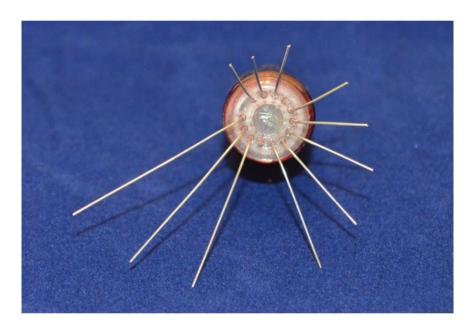
Now you can insert and solder in the tube. There are 11 leads on the trimmed tube and 12 pads on the PCB. One of the pads on the PCB is unconnected. DO NOT INSERT A LEAD INTO THIS HOLE:
