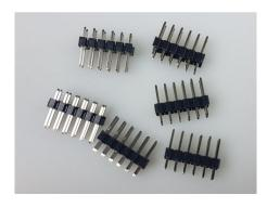
Ensure the connectors are soldered very close to the PCB. Also now insert IC3 into its socket, with the dot on the bevelled face pointing to the front of the PCB.
