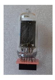
The tube cell is now complete. Repeat for the other 5 tubes. Then move on to step 6.
