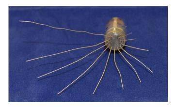
Now you can insert and solder in the tube. Insert the 12 leads into the 12 holes. Pay attention that the tube sits squarely on the PCB. Keep the tube 5mm (0.2") from the PCB. Failure to keep this separation will invalidate any tube warranty claim.
