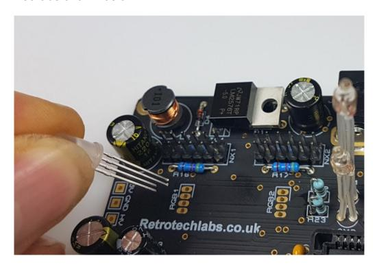
Then, place a Nixie Tube assembly into position on the 6X2 connectors. Push the RGB LED gently into position under the tube and then solder in place.
