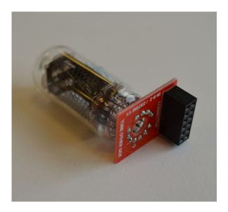
The tube cell is now complete. Repeat for the other 5 tubes. Then move on to step 6.
