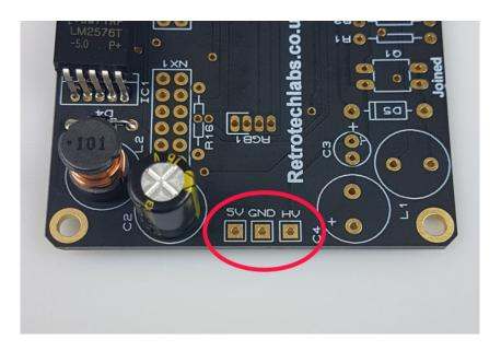
Plug in the power supply, and then test using a DC voltmeter: Touch the black probe on the GND test point and the red probe on the 5V test point. The voltage should measure between 5.6 and 5.9 Volts. If not, disconnect power and check your work. Do not proceed with the assembly until the error is corrected. Once the test is completed, disconnect the power.
