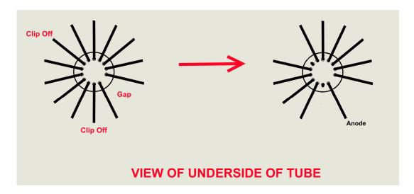
To facilitate easy insertion of the flying leads into the small holes, it helps enormously to trim the flying leads with a pair of scissors. Start at one of the leads at the back of the tube. Then, working around the tube, cut each sucessive lead approx 2mm shorter than the previous one. This will allow you to feed each lead in in turn.
