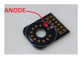
Now you can insert and solder in the tube. Pay attention that the tube sits squarely on the PCB. Then solder on the connector.
