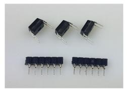
You will either receive 2 X 6 Way sockets, or a strip of 12 sockets. If the latter, clip in the middle to get two 6 way socket strips. Assemble the parts as shown below, paying attention to the orientation of the dot on the body of the parts. Then solder the sockets in place. Don't solder the parts to the sockets!
