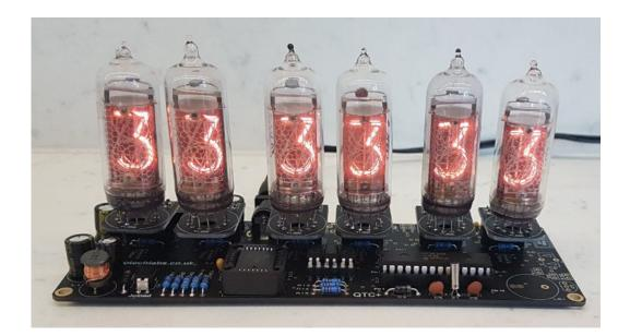
If you do not get this count up, or have missing or overlapping digits, stop and check your work. Try swapping tubes around to see if the problem is with the tube, or the location. Please make these basic tests before contacting us for help and have the results to hand.
