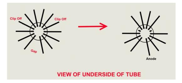
To facilitate easy insertion of the flying leads into the small holes, it helps enormously to trim the flying leads with a pair of scissors. Start at one of the leads at the back of the tube. Then, working around the tube, cut each successive lead approx 2mm shorter than the previous one. This will allow you to feed each lead in in turn.
