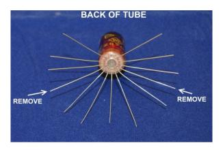
This is how the tube will look after removing the leads:
