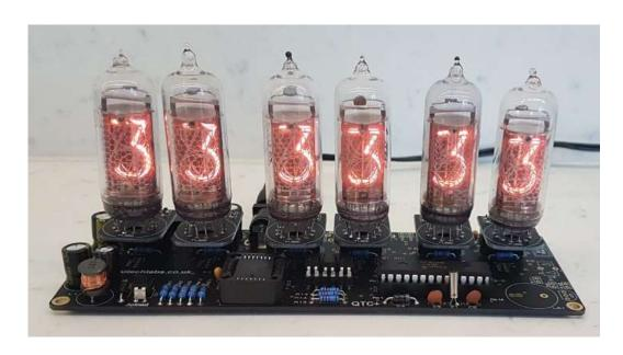
If you do not get this count up, or have missing or overlapping digits, stop and check your work. Try swapping tubes around to see if the problem is with the tube, or the location. Please make these basic tests before contacting us for help and have the results to hand.
