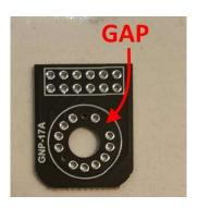
First, spread out all 13 wires equally, as shown below and you will note the gap in the wires:
