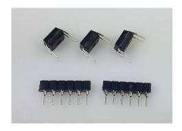
You will either receive 2 X 6 Way sockets, or a 12 way IC socket. Assemble the parts as shown below, paying attention to the orientation of the dot on the body of the parts.
