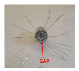
Then, working around the tube, cut each sucessive lead approx 2mm shorter than the previous one. This will allow you to feed each lead in in turn.
