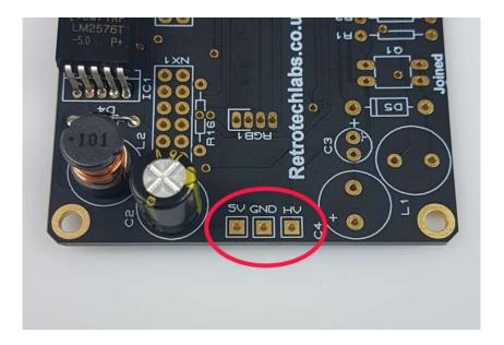
Plug in the power supply, and then test using a DC voltmeter: Touch the black probe on the GND test point and the red probe on the 5V test point. The voltage should measure between 5.6 and 5.9 Volts. If not, disconnect power and check your work. Do not proceed with the assembly until the error is corrected. Once the test is completed, disconnect the power.
