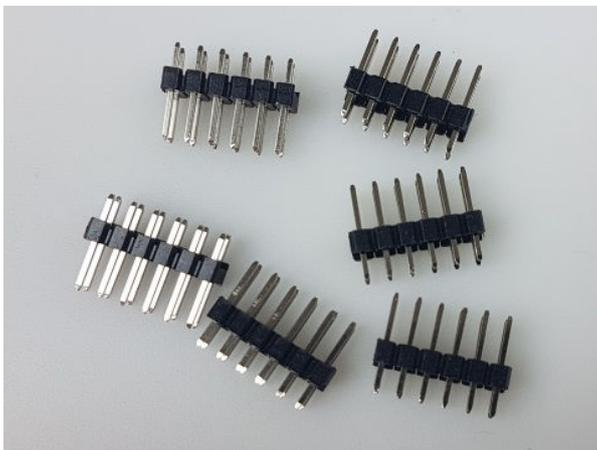
Take care that the headers are fully flush against the PCB when soldering. It helps to solder a single pin first, then check (and if necessary adjust), before soldering the remaining 11 pins.
