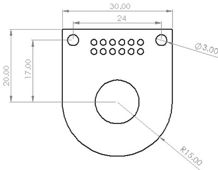
Dimensions and layout of IN-18 Cell PCB
