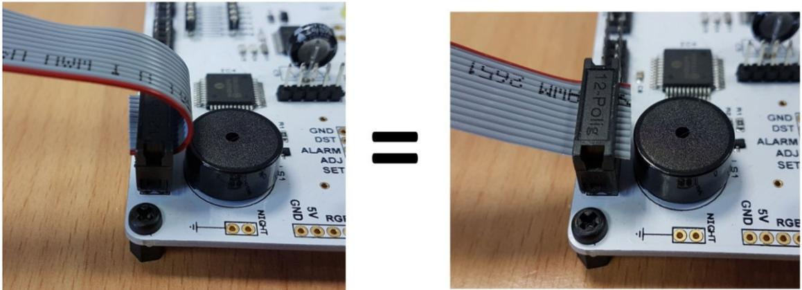
The direction the ribbon leaves the driver board does not matter
