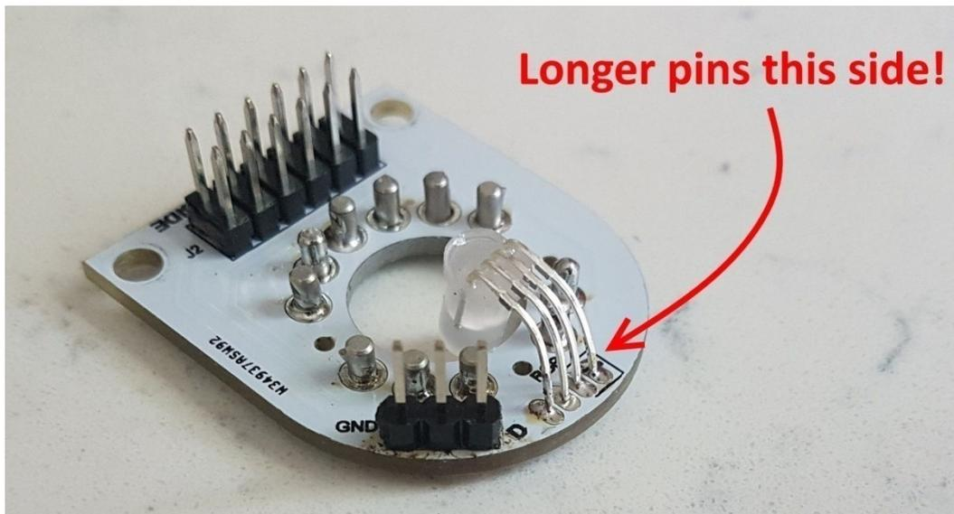
Solder the 3 way header too, as shown above. The connection to the main board is now easily made with 3 way cables as available on our website in several lengths.
