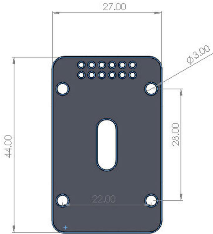
Dimensions and layout of IN-12 Cell PCB
