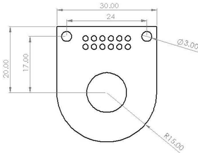
Dimensions and layout of Z5660M / ZM1040 Cell PCB
