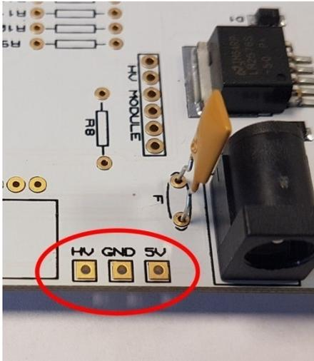
Plug in the 12V DC power supply, and then test using a DC voltmeter on 20V DC setting: Touch the black probe on the GND test point and the red probe on the 5V test point. The voltage should measure between 4.9 and 5.2 Volts. If not, disconnect power and check your work. Do not proceed with the assembly until the error is corrected. Once the test is completed, disconnect the power.
