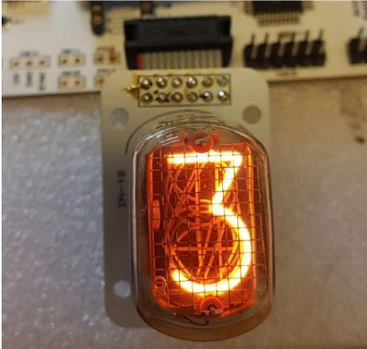
Use the tube and connector assembly to check that each digit shows at each location from NX1 to NX6. Power off the board each time as you switch the tube between locations.
