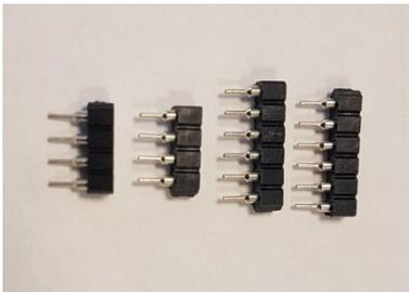
We have chosen to provide sockets for these resistors, to allow flexibility of design so that users can change tube type easily and experiment with different anode resistors to get the brightness they want from the tubes. No desoldering / soldering is necessary to change the resistors!
