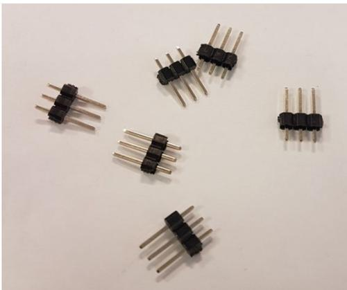
Now place the headers into the PCB and secure with the 6X2 Female connector. It will hold them perfectly in place whilst you solder all 18 pads. It has no other purpose – it is just a jig to hold all the pins in position whilst you solder the pads.
