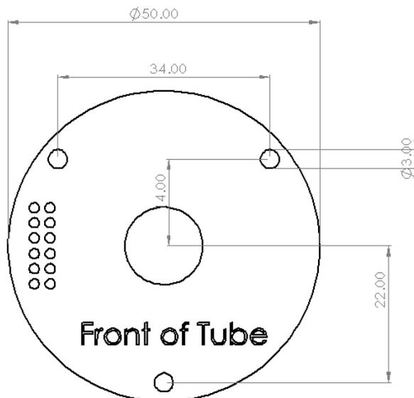
Dimensions and layout of R|568M Cell PCB
