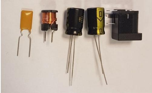
C1 and C2 are polarized. The positive lead is the longest, and goes in the pad marked '+'.
