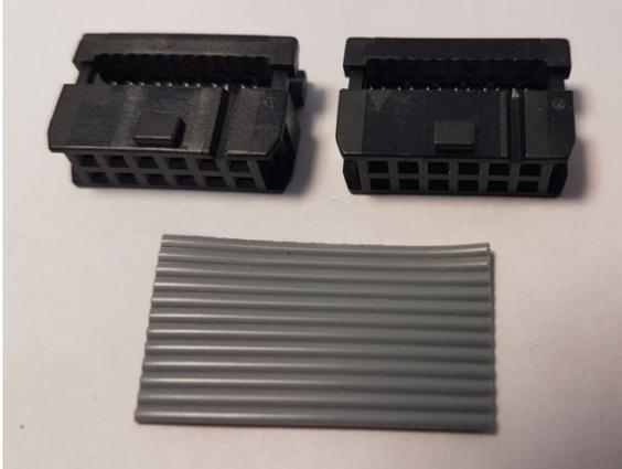
Using a pair of pliers or a plumber's wrench (or, even better the correct tool for these connectors!). crimp one connector to one end of the cable:
