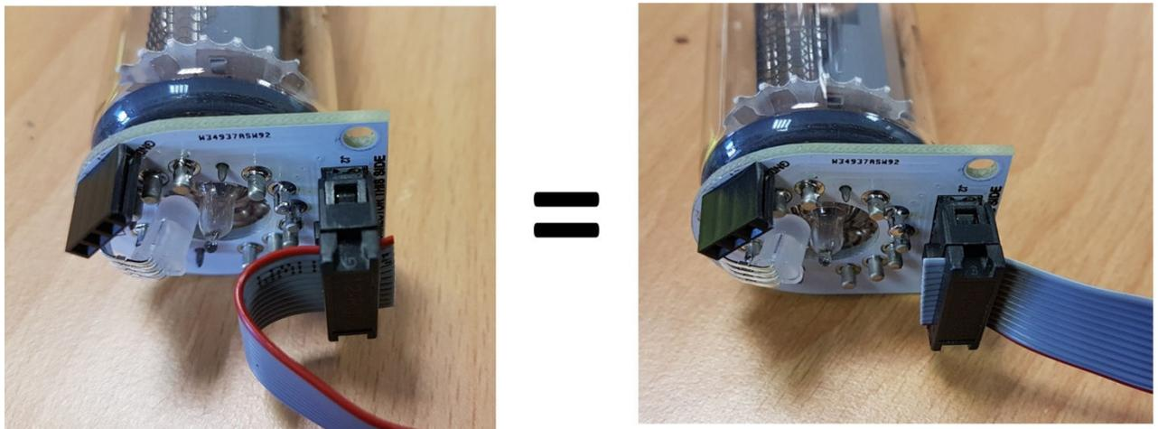
Also note that the IDC connectors may face the same direction or in opposition, it does not matter. Plan what is best for YOUR installation:
