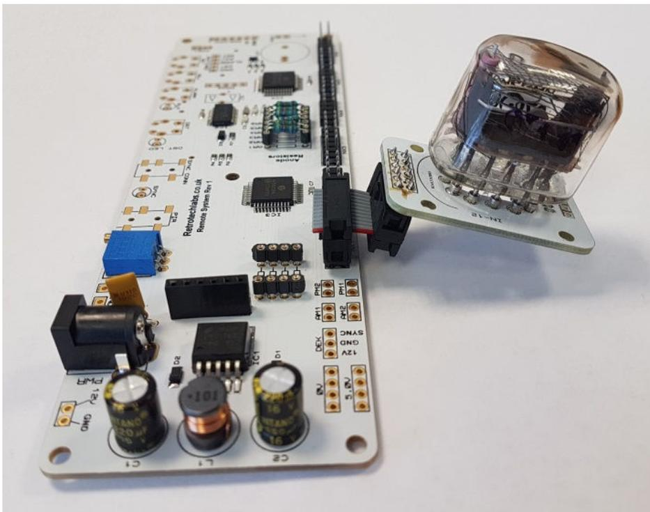
Insert again the HV Module, and now taking care that high voltage will be present on the PCB, power up the board. After a short pause, the tube should start counting 0 through to 9 and repeating.
