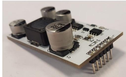
First solder the Male header to the PCB Module as shown above.
