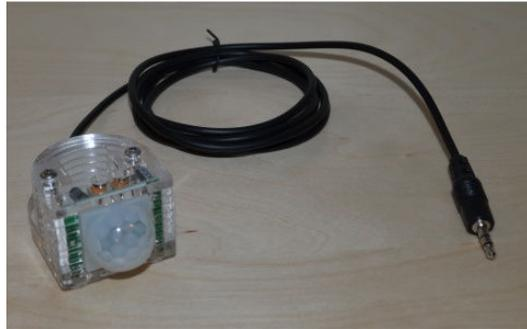
When installed and configured (configuration parameter 17), the sensor will sense motion in the room, and switch off the High Voltage generator, tubes and RGB LEDs when the PIR time period has expired.
