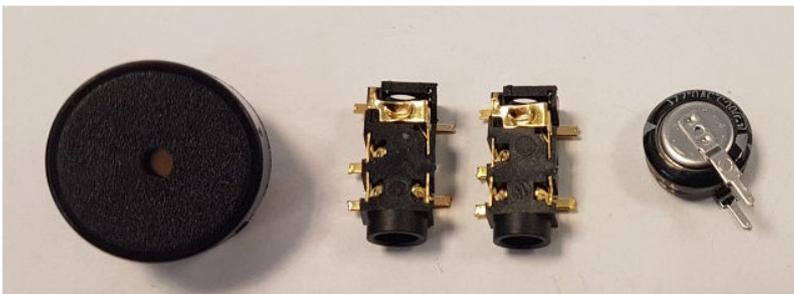
The 0.22F capacitor is polarised – note the arrows on the PCB, to correspond with the arrows on the part.
