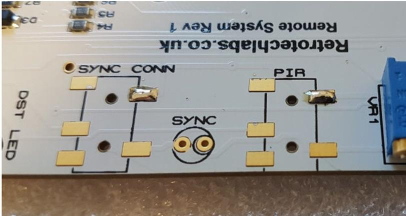
Then place the socket over the pad and re-heat the pad to wet the solder and anchor the part. The remaining pads can then be soldered.
