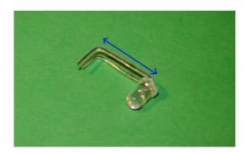
The six LEDs may now be installed, as shown below. Insert and solder on the COMPONENT side. Take care that the LED leads are well clear of the tube leads:
