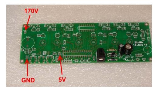
Plug in the power supply, and then test using a DC voltmeter: Touch the black probe on the GND test point and the red probe on the 5V test point. The voltage should measure between 5.1 and 5.3 Volts. If not, disconnect power and check your work. Do not proceed with the assembly until the error is corrected. Once the test is completed, disconnect the power.
