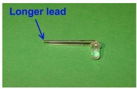
Now bend again, appropriate to the spacing between the pads for the LED and the hole for the LED. Cut the leads to the same length:
