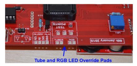
Shorting the two 'RGB' pads will switch off the RGB LEDs.
