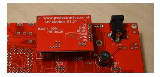
Nixie Tube Clock 'Spectrum 18' Issue 4 (20 August 2015) www.pvelectronics.co.uk Later, at the end of the assembly, when the clock is ready to be put into its case you can use the small adhesive dot on the top of the HV Module's 4.7uF 250V capacitor to stick it to the bottom of the PCB to keep it from moving. Do this later.
