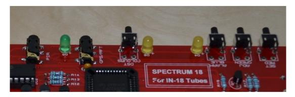
To solder the GPS / RFT and PIR connectors: First wet one pad on the PCB with solder. Then place the connector in position and retouch the pad with the soldering iron. This will anchor the component and then you can solder the remaining pads.
