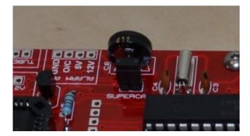
Note: C6 and the 2 Way jumper need to be soldered on the bottom side of the PCB if you are mounting the clock in the Visio case.
