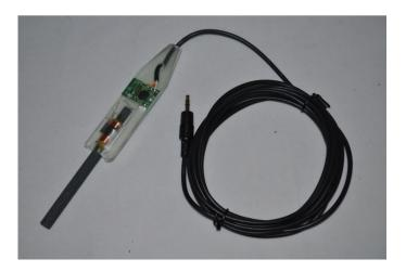
**DCF Module:** For receiving time signals from transmitter at Frankfurt, Germany. Reception is possible within a 2000Km radius of Frankfurt.
