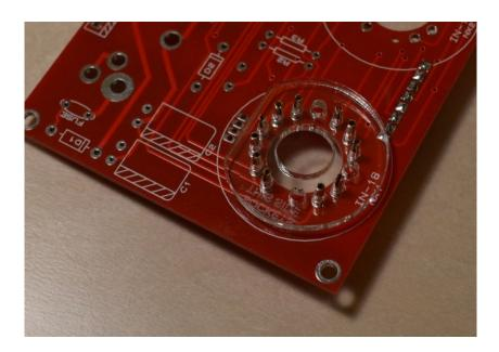
After soldering all 66 contacts, clip off the lower, very thin part of the connector.
