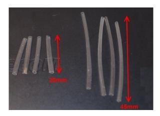
Slip the insulation over the neon lamp leads and with a hot air gun, shrink the tubing:
