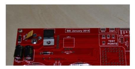
Plug in the power supply, and then test using a DC voltmeter: Touch the black probe on the GND test point and the red probe on the 5V test point. The voltage should measure between 4.8 and 5.2 Volts. If not, disconnect power and check your work. Do not proceed with the assembly until the error is corrected. Once the test is completed, disconnect the power.
