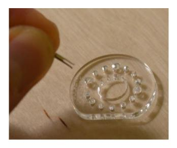
Push all the sockets firmly into place until they stop. You will end up with 6 socket assemblies. Put them to one side. Do not solder them to the PCB yet.
