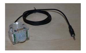
When installed and configured (configuration parameter 17), the sensor will sense motion in the room, and switch off the High Voltage generator, tubes and RGB LEDs when the PIR time period has expired.
