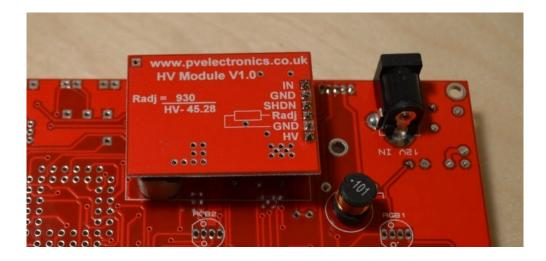
Later, at the end of the assembly, when the clock is ready to be put into its case you can use the small adhesive dot on the top of the HV Module's 4.7uF 250V capacitor to stick it to the bottom of the PCB to keep it from moving. Do this later.
