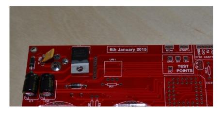
Plug in the power supply, and then test using a DC voltmeter: Touch the black probe on the GND test point and the red probe on the 5V test point. The voltage should measure between 4.8 and 5.2 Volts. If not, disconnect power and check your work. Do not proceed with the assembly until the error is corrected. Once the test is completed, disconnect the power.
