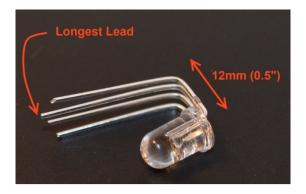
If you follow the bending instructions above, then the longest lead should go into the hole marked with 2 small circles at each RGB LED location. Solder each LED and clip the leads short.
