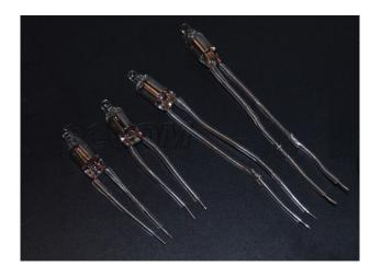
Finally, solder the neons in place on the PCB, with the taller neons at the back. The glass cover tubes can be placed over later.
