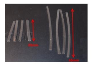
Slip the insulation over the neon lamp leads and with a hot air gun, shrink the tubing:
