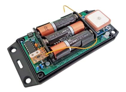
Additional data is transmitted such as battery voltage and GPS fix time.
