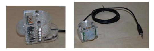
When installed and configured (configuration parameter 17), the sensor will sense motion in the room, and switch off the High Voltage generator, tubes and RGB LEDs when the PIR time period has expired.
