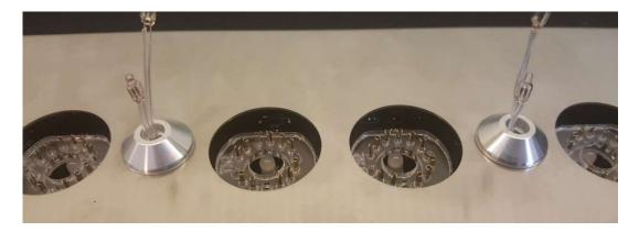
The two glass neon cover tubes can now be placed, however it's a good idea to insert the tubes first. The glass covers can be sealed with a tiny drop of silicone sealant, but this prevents easy disassembly – we recommend they are held in place solely by gravity!
