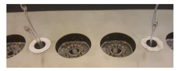
Then peel the upper protective layer from the adhesive circles, to reveal the clear adhesive film. Slide the tower bases over the neons and press firmly into the adhesive.
