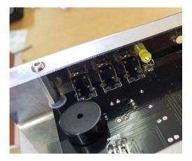
When the LEDs are in their holes, you can remove the screws but do not allow the PCB to move with respect to the case, or the LEDs will come out of their holes. If you grip the assembly as shown below, you can keep the PCB in the correct position whilst you remove the screws and move to the next step:
