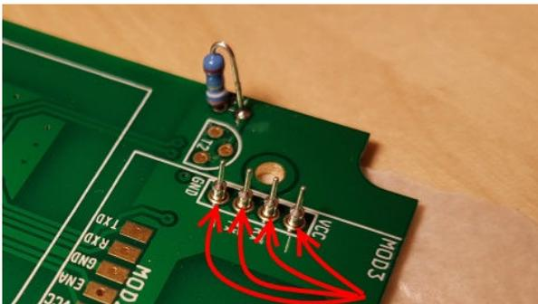
Now plug the four way header strip over the pins and also screw on the 6mm spacer as shown below, using a M3 X 4mm plastic screw.
