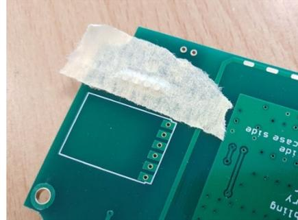
Flip over the PCB and solder the four sockets with minimal solder, as shown below. As soon as you see the solder flow around the annulus, you can withdraw the solder and iron.
