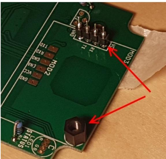
Now place on the GPS assembly, over the four connector pins and screw in place with the other M3 X 4mm plastic screw, then solder the four pins to the GPS. Keep the GPS level and pushed down as you solder.
