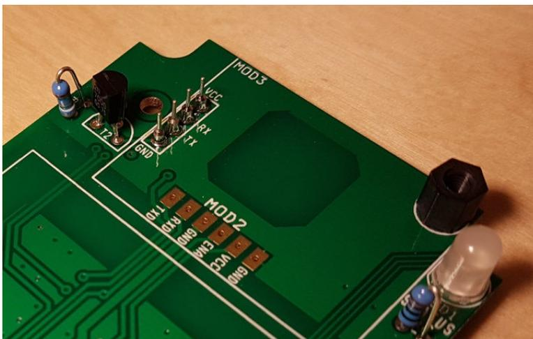
The longest lead of the LED goes in the marked hole. Take care you orient correctly.
