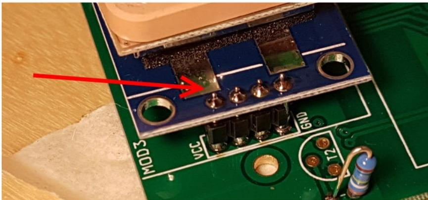
Once the pins have been soldered, unscrew the top plastic screw and withdraw the GPS. Don't forget to put it back again later!
