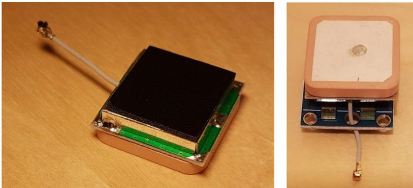
Now clip the antenna connector into the small matching connector on the component side of the GPS module. It helps to press with a hard surface, such as a small block of metal.
