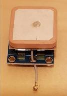
Now clip the antenna connector into the small matching connector on the component side of the GPS module. It helps to press with a hard surface, such as a small block of metal.
