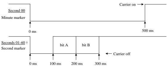
Two bits, numbered xxA and xxB for second xx bit polarity: 0=on, 1=off
