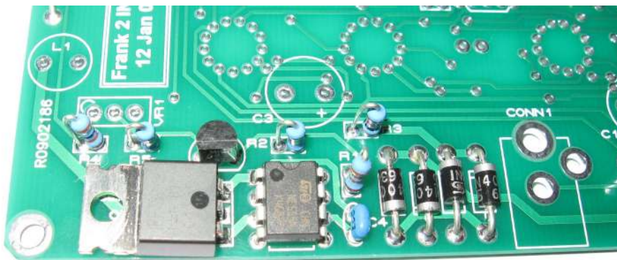
Figure 8: R1 to R5 placed vertically
