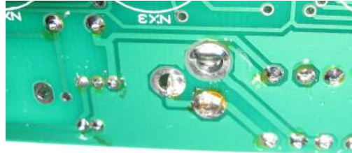
Figure 14: Underside view of CONN1
