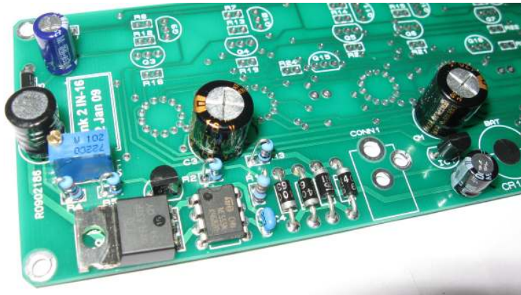
Figure 12: Electrolytic capacitors placed on the PCB
