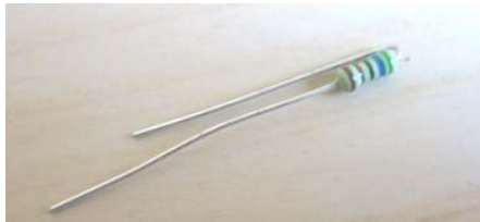
Figure 7: Resistor leads formed for mounting upright.
