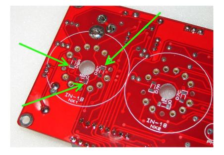
Now identify the cathode mark on the LEDs. This is usually a green marking at one end of the LED, though it may be under the LED lens and harder to see, It may also be an arrow or a line pointing in one direction on the underside of the LED:
