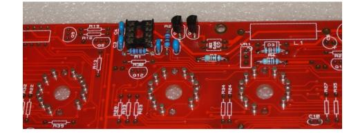
4.5 Q3 - IRFD220 D3 - UF4004 L1 - Inductor C5 - 470μF C8 - 1μF VR1 - 1K Pot
