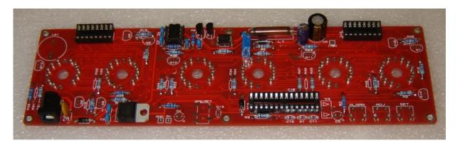
4.9 Q5, Q6, Q7, Q11, Q12, Q13 (all MPA42) Q8, Q9, Q10 (all MPSA92)
