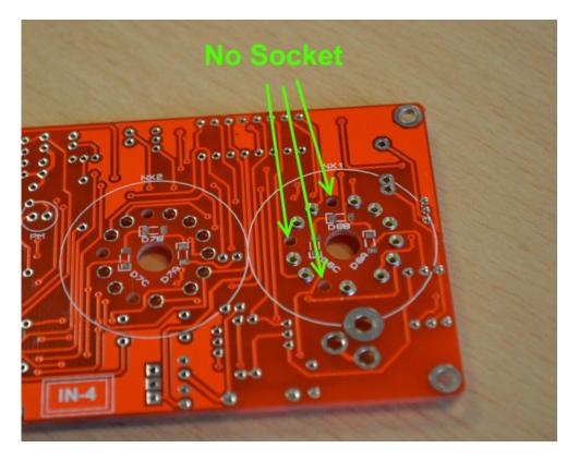
Be sure to insert the sockets FROM the tube side of the PCB – the side with the tube markings.
