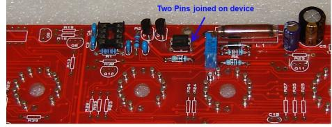
Take care that the two pins that are joined go in the position marked. C5 and C8 are polarised. The longer lead goes in the +' hole.
