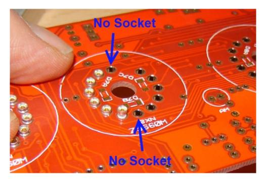
Be sure to insert the sockets FROM the tube side of the PCB – the side with the tube markings.
