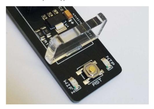
**5.** Push the ESP module into place in the 4X2 header and it should sit in the recess of the plexi support.
