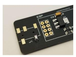
Then place the connector in position and re-touch the pad with the soldering iron whilst pressing the connector onto the PCB. This will anchor the component and then you can solder the remaining pads.
