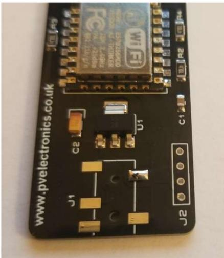
Then place the connector in position and re-touch the pad with the soldering iron whilst pressing the connector onto the PCB. This will anchor the component and then you can solder the remaining pads.
