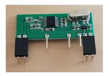
Then position on the PCB. Press the black connectors level with the the PCB, and check alignment of the module before soldering the four pads. Then withdraw the CY18 module until later.
