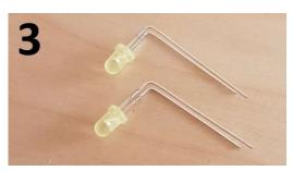
Now the anode leads of the LEDs will be in the correct orientation as you insert into the holes in the PCB behind the ALARM and DST switches. Use the jig again, to align the LEDs above the switches. This will give the correct spacing for if you want to use one of our cases.
