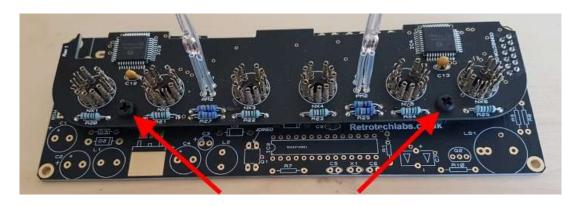
You can now solder the 12 way connector, on the bottom of the driver PCB. Then remove the tube PCB and all the screws and spacers.
