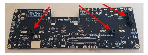
Then place the tube PCB in position, and engage the 12 way connectors and screw together with the longer 5mm screws.
