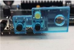
Now bend and solder D7. The longer lead goes in the pad with a circle around it. Think about the orientation before you bend the leads. D7 should be level with the GPS jack socket next to it, and protrude by its full body length from the rear of the PCB.
