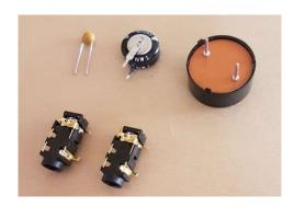
The 0.22F capacitor is polarised – note the arrows on the PCB, to correspond with the arrows on the part. To solder the SMD jack sockets, first tin one pad per jack socket:
