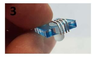
Then install the RGB LEDs from the base of the PCB.
