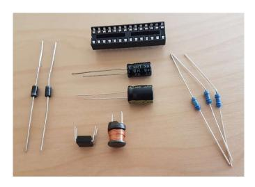
Take care that the notched end of the IC socket is at the end shown. However if after you solder the part you realise the notch is at the wrong end, DON'T try to desolder it! Actually, so long as the IC has the correct orientation, the socket does not really matter. Also the MOSFET needs to be placed with the two joined pins as marked on the PCB.
