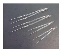
NOTE: If you will be using our Oak, Walnut or Plexi Case, to allow clearance for the neon cover tubes, only use one piece of insulation on the taller neons – leave the other lead without insulation Finally, solder the neons in place on the PCB, with the taller neons at the back. The glass cover tubes can be placed over later.
