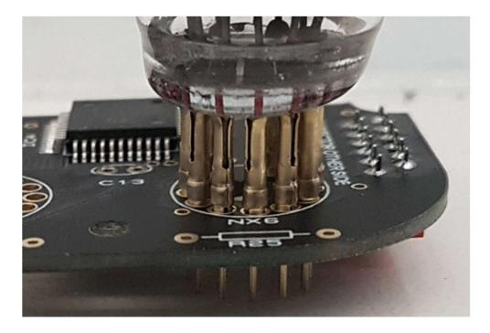
Flip over the PCB and solder the pins, ensuring the tube stays vertical. Solder sparingly – as soon as you see solder flow around the annulus, withdraw the solder and soldering iron.
