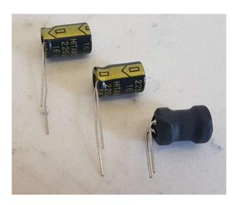
Then solder these three parts noting that the inductor L1 is placed on the opposite side of the PCB to the capacitors C1 and C2.
