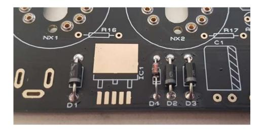
IC1 is a Surface Mount part, but it is large and easy to solder. Start by wetting one pad with solder. Then place the part in position and heat the lead so the solder below it melts and anchors the part. The four other leads can then be soldered. Do not solder the heatsink tab.
