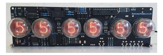
If you do not get this count up, or have missing or overlapping digits, stop and check your work. Try swapping tubes around to see if the problem is with the tube, or the location. Please make these basic tests before contacting us for help and have the results to hand.
