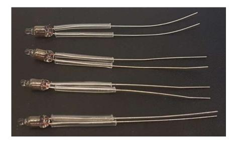
Finally, solder the neons in place on the PCB. Its easier to solder one pad of the neon first, then make adjustments to make sure it is perpendicular, before soldering the second pad.
