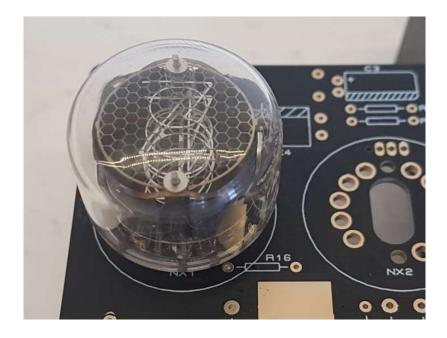
Then flip over the PCB and solder the 11 sockets in place, then remove the tube.
