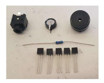
The jack socket, piezo buzzer and C8 are mounted on the back of the PCB. Ensure the arrows on C8 are aligned with the corresponding arrows on the PCB
