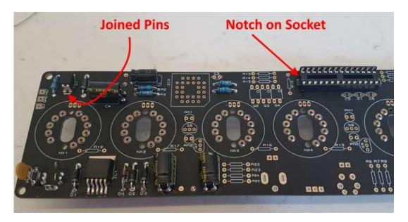
Take care that the notched end of the IC socket is at the end shown. However, if you find you soldered it with the wrong orientation, do not try to remove it. It is perfectly fine with the notch at the wrong end, just be sure to place the IC in the socket with the IC's notch in the correct position.
