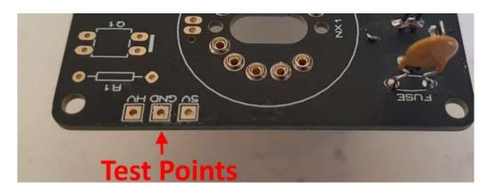
Plug in the power supply, and then test using a DC voltmeter: Touch the black probe on the GND test point and the red probe on the 5V test point. The voltage should measure between 5.4 and 5.8 Volts. If not, disconnect power and check your work. Do not proceed with the assembly until the error is corrected. Once the test is completed, disconnect the power.
