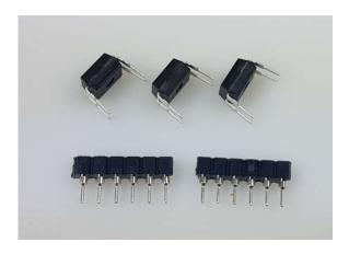
You will either receive 2 X 6 Way sockets, or a 12 way IC socket. Assemble the parts as shown below, paying attention to the orientation of the dot on the body of the parts.
