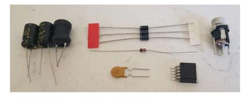
Start by installing D1-D4. The diodes are polarized – the band on the part must match the band marked on the white PCB marking.
