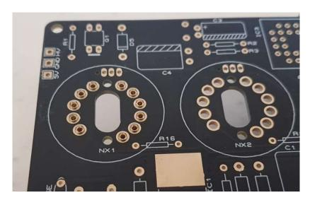
After inserting the sockets, the best way to hold all the sockets in place whilst soldering them is to insert a tube.
