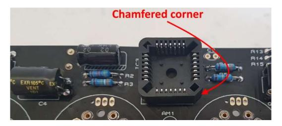
Now insert IC3, with the dot and chamfered edge aligned as shown by the arrow in the picture below.
