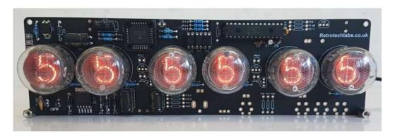
If you do not get this count up, or have missing or overlapping digits, stop and check your work. Try swapping tubes around to see if the problem is with the tube, or the location. Please make these basic tests before contacting us for help and have the results to hand.
