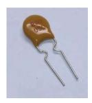
The 22pF and 47pF capacitors will be marked 22 or 220 and 47 or 470 respectively. The 100nF capacitors will be marked 104.
