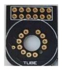
These tubes have 2 leads that need to be removed as shown below. Use the gap to correctly orient the tube:
