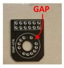
Note the gap in the circle of holes, which matches up with the gap in wires on the tube. Also note there are 2 holes which have no solder pad – these are for unused wires so the wires should be inserted and then clipped off.
