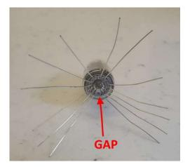
Then, working around the tube, cut each sucessive lead approx 2mm shorter than the previous one. This will allow you to feed each lead in in turn.
