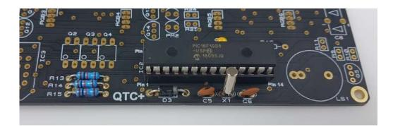
4.7 Q2, Q3, Q4 (EL817) SIL Socket Strip or IC sockets
