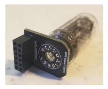
Now you can insert and solder in the tube. Insert the 11 leads into the 11 holes. Pay attention that the tube sits squarely on the PCB. **Keep the tube 5mm (0.2") from the PCB. Failure to keep this separation will invalidate any tube warranty claim.**
