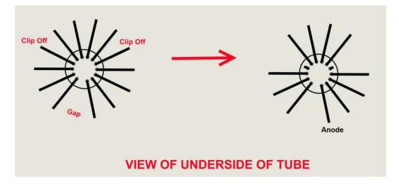
To facilitate easy insertion of the flying leads into the small holes, it helps enormously to trim the flying leads with a pair of scissors. Start at one of the leads at the back of the tube. Then, working around the tube, cut each successive lead approx 2mm shorter than the previous one. This will allow you to feed each lead in in turn.
