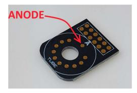
Now you can insert and solder in the tube. Pay attention that the tube sits squarely on the PCB. Then solder on the connector. Keep the tube 5mm (0.2") from the PCB. Failure to keep this separation will invalidate any tube warranty claim.
