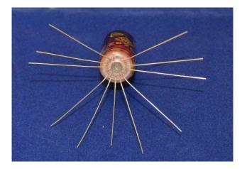
To facilitate easy insertion of the flying leads into the PCB holes, it helps enormously to trim the remaining flying leads with a pair of
