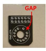
First, spread out all 13 wires equally, as shown below and you will note the gap in the wires:
