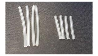
**NOTE**: If you will be using our Oak, Walnut or Plexi Case, to allow clearance for the neon cover tubes, only use one piece of insulation on the taller neons – leave the other lead without insulation Slip the insulation over the neon lamp leads and with a hot air gun, shrink the tubing:
