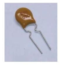
The 22pF and 47pF capacitors may be marked 22 and 47 or 220 and 470 respectively. The 100nF capacitors will be marked 104.
