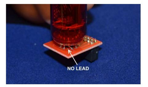
Insert from the side of the PCB with no markings. Pay attention that the tube sits squarely on the PCB. Then solder on the connector.
