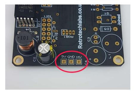
Plug in the power supply, and then test using a DC voltmeter: **Nixie Tube Clock 'Nixie QTC+' Issue 4 (13 Feb 2023)** www.pvelectronics.co.uk Touch the black probe on the GND test point and the red probe on the 5V test point. The voltage should measure between 5.6 and 5.9 Volts. If not, disconnect power and check your work. Do not proceed with the assembly until the error is corrected. Once the test is completed, disconnect the power.
