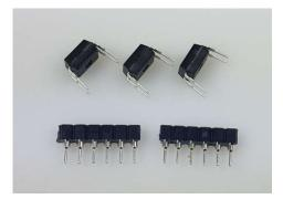
You will either receive 2 X 6 Way sockets, or a 12 way IC socket , or two 6 way IC sockets. Assemble the parts as shown below, paying attention to the orientation of the dot on the body of the parts.
